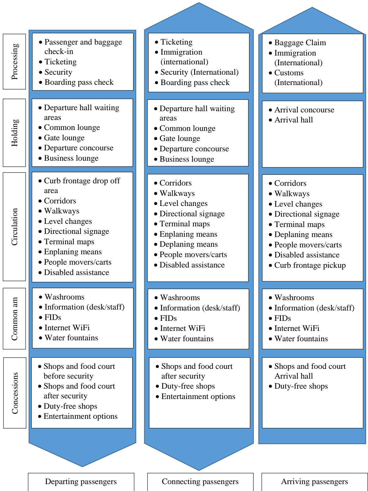
Figure 3-6: Overall service environment
